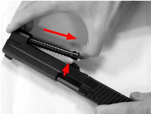
REMOVE THE RECOIL SPRING GUIDE AND SPRING.
