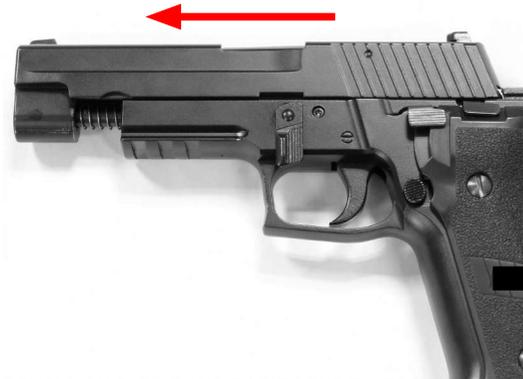
REMOVE MAGAZINE AND ROTATE THE TAKEDOWN LEVER CLOCKWISE UNTIL IT STOPS AND REMOVE THE SLIDE.
